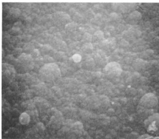
FIG. 2. SEM photographs of the poly-T26P film. (a): Electrode side (3000X). (b): Solution side (3000X). (c): Cross section (4000X). Thickness: 10 \mu\text{m} .
